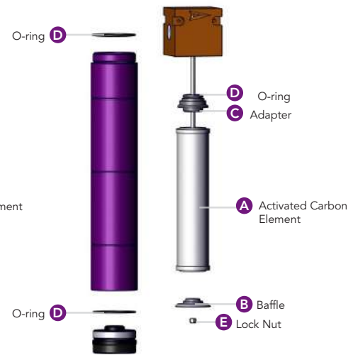
Figure 5 : Activated Carbon Filter
