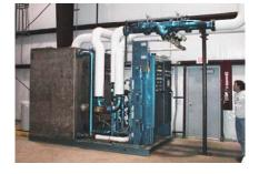
STRAINERS WITH AUTOMATIC BLOWDOWN: This OE type system has a Stainless Steel coldwell and automated strainers. Pressure differential is monitored across the strainers. When the preset trip pressure is reached, automated valves open and flush the strainers for a preset period of time.
