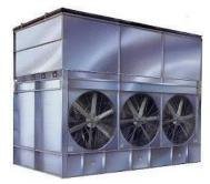
Closed-circuit evaporative cooler. The evaporative-type heat exchanger utilizes heavy-duty prime surface evaporator coils to circulate the heated process coolant through a cascading water spray. The spray, atomized over coils by an upward air flow, transfers heat quickly and cleanly. A thermostatically controlled pump then recirculates water from the sump to the spray nozzles. Automatic thermostatic dampers provide accurate, continuously varying capacity control. The dampers
